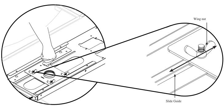
**Step 3.** Determine final placement of the upper adapter plate.
